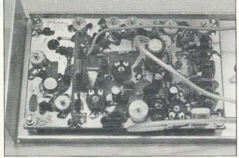
Photo. The 1-watt ATV transmitter.
